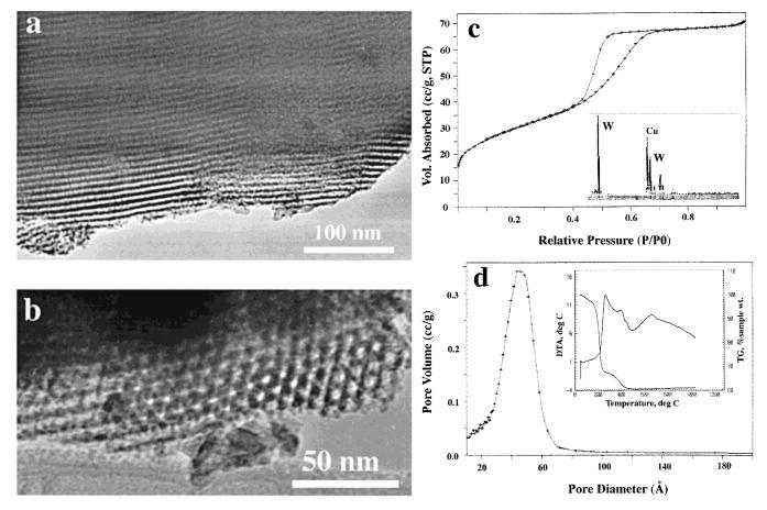
**Figure 11.** (a and b) TEM micrographs of two-dimensional hexagonal mesoporous  $WO_3$  recorded along the [110] and [001] zone axes. (c and d) Nitrogen adsorption–desorption isotherms and BJH pore size distribution plot for calcined  $WO_3$ . Inset in part c is the corresponding EDX spectrum, and in part d the TGA trace obtained on the as-synthesized W(O,CI)/copolymer composite.
