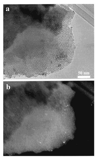
**Figure 6.** (a) Bright-field TEM image of a thin slice of the hexagonal mesoporous  $ZrO_2$  sample. (b) Dark-field image obtained on the same area of the same  $ZrO_2$  sample. The bright spots in the image correspond to  $ZrO_2$  nanocrystallites.
