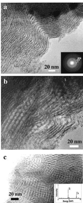
**Figure 2.** TEM micrographs of two-dimensional hexagonal mesoporous  $TiO_2$  recorded along the (a) [ll0] and (b) [001] zone axes, respectively. Inset in part a is selected-area electron diffraction patterns obtained on the image area. (c) TEM image of cubic mesoporous  $TiO_2$  accompanied by the corresponding (inset) EDX spectrum acquired for this sample.
