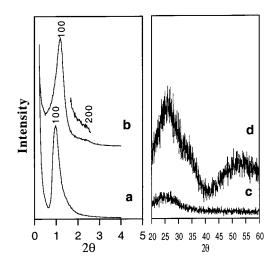
Figure 7. Low-angle and wide-angle X-ray diffraction (XRD) patterns of (a and c) as-synthesized Nb(O,Cl)/ $EO_{20}PO_{70}EO_{20}$  composite mesostructure and (b and d) calcined mesoporous Nb<sub>2</sub>O<sub>5</sub>.
