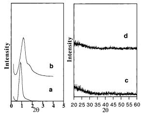
**Figure 13.** Low-angle and wide-angle X-ray diffraction (XRD) patterns of (a and c) as-synthesized (Si,Ti)(O,Cl)/ $EO_{20}PO_{70}EO_{20}$  composite mesostructure and (b and d) calcined mesoporous SiTiO<sub>y</sub>.
