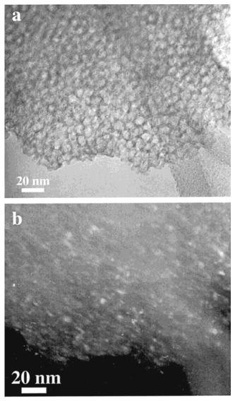
**Figure 3.** (a) Bright-field TEM image of a thin slice of the hexagonal mesoporous  $TiO_2$  sample. (b) Dark-field image obtained on the same area of the same  $TiO_2$  sample. The bright spots in the image correspond to  $TiO_2$  nanocrystallites.
