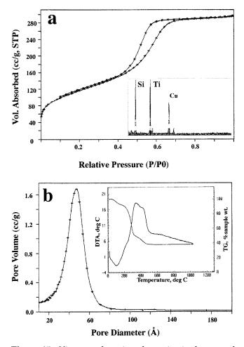
**Figure 15.** Nitrogen adsorption–desorption isotherms and BJH pore size distribution plot for calcined SiTiO<sub>y</sub>. Inset in part a is the EDX spectrum taken on the calcined sample; inset in part b is the TGA trace obtained for the as-synthesized sample.
