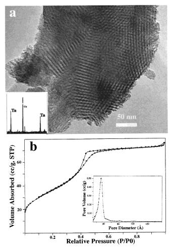
**Figure 9.** (a) TEM micrograph of two-dimensional hexagonal mesoporous  $Ta_2O_5$  recorded along the [001] zone axis. The corresponding EDX spectrum is shown in the inset. (b) Nitrogen adsorption–desorption isotherms and BJH pore size distribution plot (inset) for calcined  $Ta_2O_5$ .
