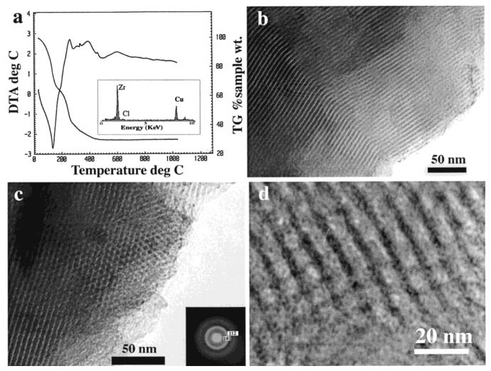
**Figure 5.** (a) TGA trace recorded for the as-synthesized  $Zr(O,Cl)/EO_{20}PO_{70}EO_{20}$  composites. (b and c) TEM micrographs of twodimensional hexagonal mesoporous  $ZrO_2$  recorded along the [ll0] and [001] zone axes, respectively. Inset in part c is selected-area electron diffraction pattern obtained on the image area. (d) TEM image of cubic mesoporous  $ZrO_2$ .
