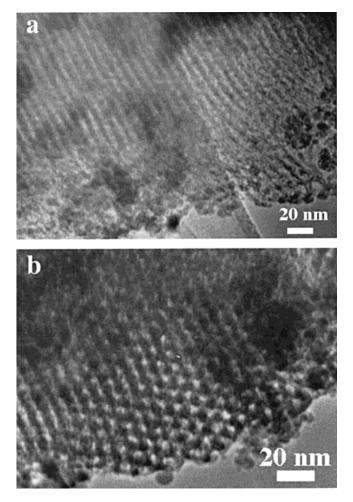
Figure 10. TEM micrographs of two-dimensional hexagonal mesoporous  $SnO_2$  recorded along the [110] (a) and [001] (b) zone axes.
