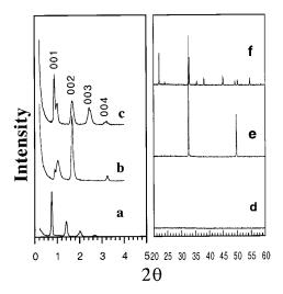
**Figure 16.** Low-angle and wide-angle X-ray diffraction (XRD) patterns of as-made Cu (O,Cl) (a and d), Mn(O,Cl) (b and e), and Cr(O,Cl) (c and f)  $/EO_{20}PO_{70}EO_{20}$  composite mesostructures.
