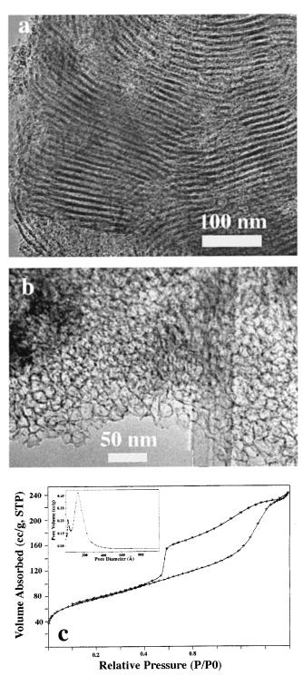
**Figure 12.** (a and b) TEM micrographs of mesoporous  $Al_2O_3$ . (c) Nitrogen adsorption–desorption isotherms and BJH pore size distribution plot (inset) for calcined  $Al_2O_3$ .
