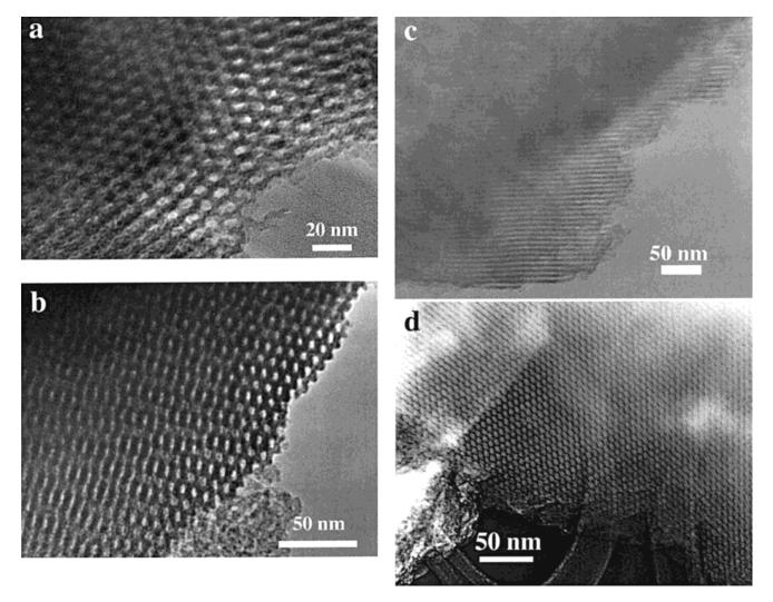
**Figure 14.** (a and b) TEM micrographs of two-dimensional hexagonal mesoporous SiTiO<sub>y</sub> recorded along [001] zone axes. (c and d) TEM micrographs of two-dimensional hexagonal mesoporous SiAlO<sub>y</sub> recorded along the [110] and [001] zone axes, respectively.
