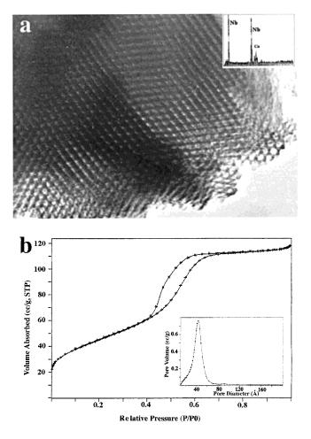
**Figure 8.** (a) TEM micrograph of two-dimensional hexagonal mesoporous  $Nb_2O_5$  recorded along the [001] zone axis. The corresponding EDX spectrum is shown in the inset. (b) Nitrogen adsorption–desorption isotherms and BJH pore size distribution plot (inset) for calcined  $Nb_2O_5$ .
