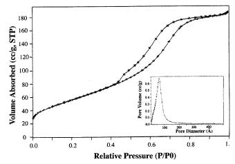
**Figure 4.** Nitrogen adsorption–desorption isotherms and BJH pore-size distribution plot (inset) for calcined cubic mesoporous TiO<sub>2</sub>.
